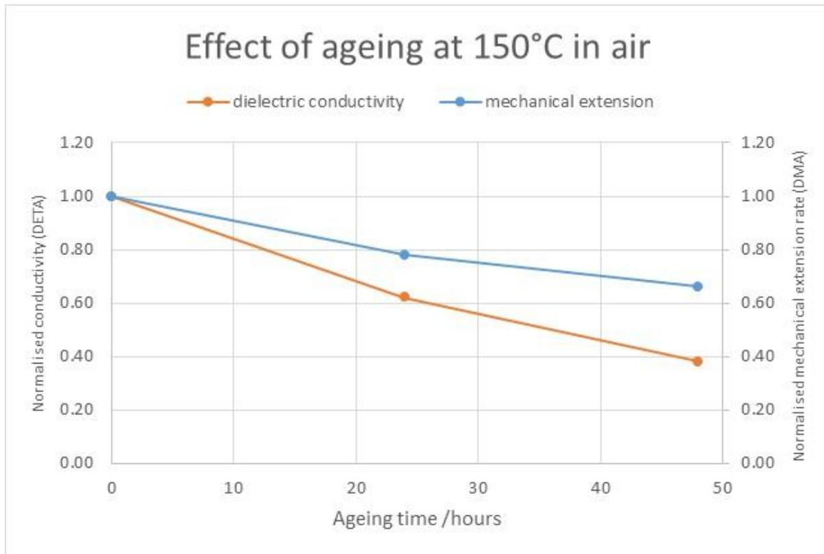
Fig 1 Effect of thermal ageing at 150°C in air for Sumac leather, as measured by the normalised conductivity and normalised mechanical extension rate. Normalised with respect to untreated, unaged sample. Samples were subjected to a controlled humidity environment (see text for details).
