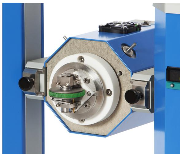
As in DMA,  $\tan \delta$  is the ratio of the loss factor ( $e''$ ) to the storage component ( $e'$ , dielectric constant or permittivity).  $\tan \delta$  is plotted against temperature and glass transition is normally observed as a peak since the material will absorb energy as it passes through the glass transition. The size of this peak quantifies the amount of amorphous material present in the sample
